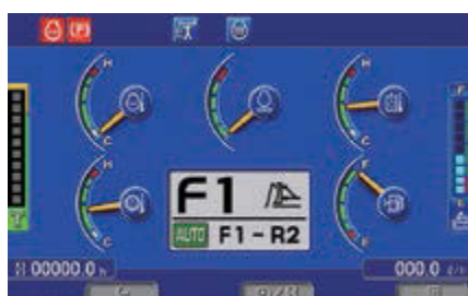
Automatic gearshift mode to further reduce fuel consumption
