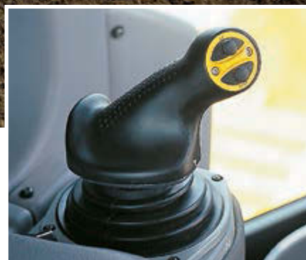
Palm Command Control System (PCCS)
