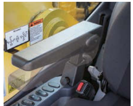
Armrest with simple height adjustment
