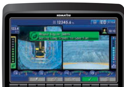
Eco-gauge, Eco guidance and fuel consumption gauge
