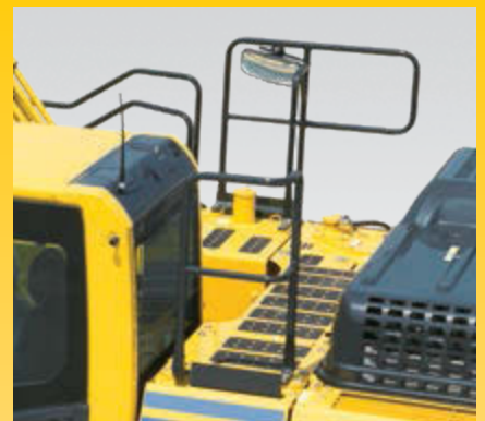
Hand rails and anti-slip plates
